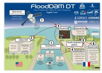
Federated Earth System Digital Twin solution between NASA IDEAS and SCO FloodDAM (Flood Detection Alert and Maping) for alert systems and flood risk maps on local and global scales using space technologies focused on flooding.
